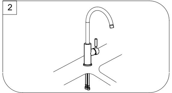
Place optional Flange at the bottom of the new faucet before positioning faucet through mounting hole.
