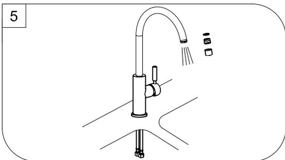
Important: After installation is completed. Turn on water supply and allow both hot and cold water to run for at least one minute each. While water is running, check for leaks. Reinstall Spray head. Your new faucet is now ready to use.
