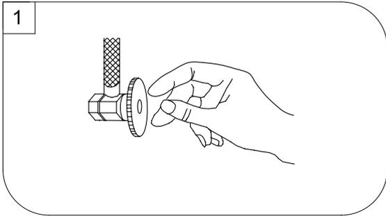
Shut off water supplies. Remove old faucet. Clean sink surface in preparation for the new faucet.
