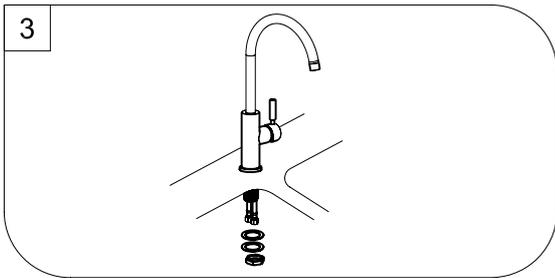
Screw the mounting stud into the body. Secure the faucet to the sink by installing plastic washer, steel washer and nut onto it. Tighten with wrench.
